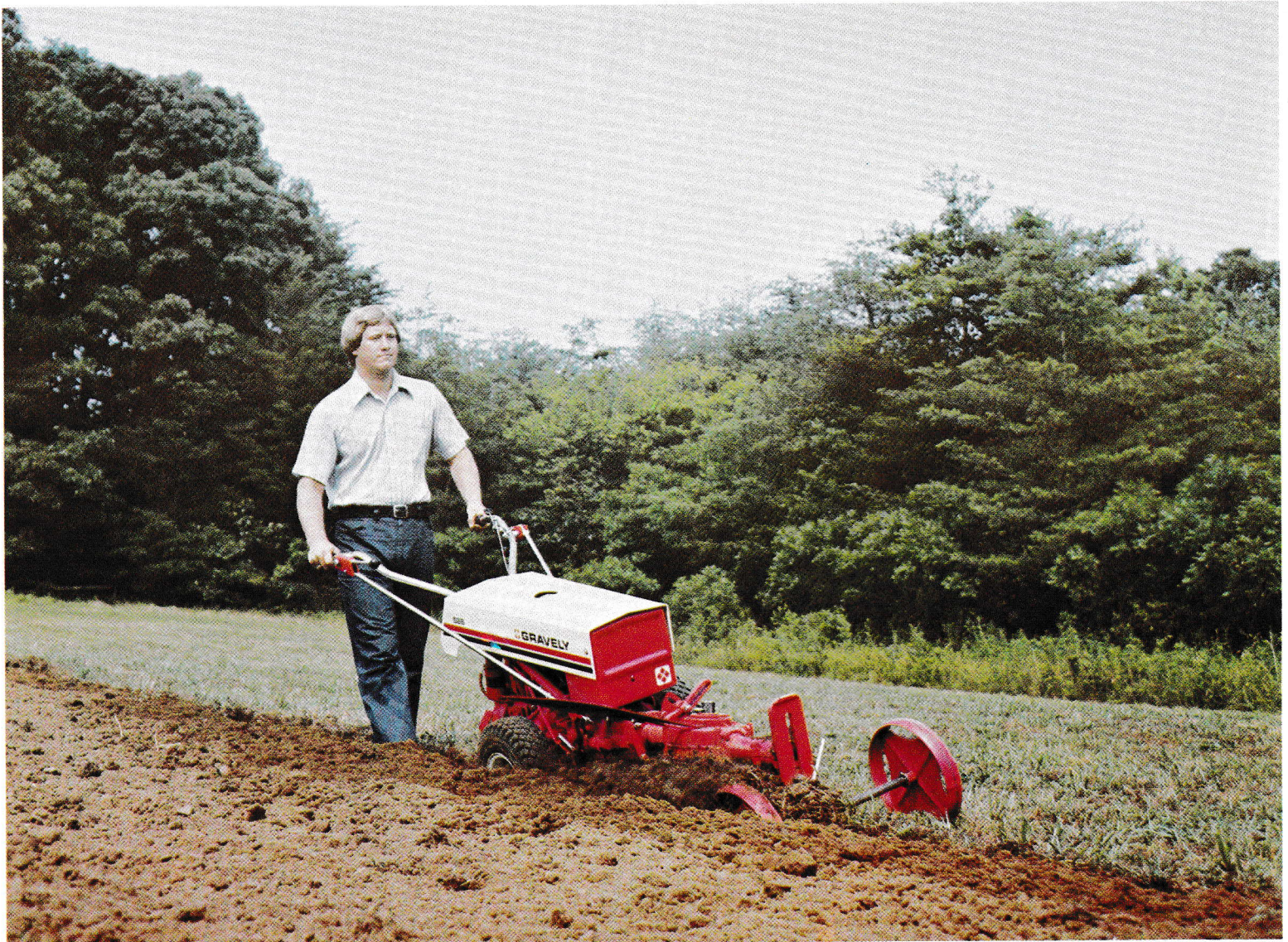
Gravely 526, 8 HP, 4-speed, electric start Convertible Tractor. Also available Model 522, electric start, 2-speed.
